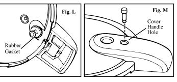
4. The overpressure plug can also be removed for cleaning by pushing it out of its opening from the top of the cover handle. After cleaning, reinsert it by pushing the domed side of the plug into the opening from the underside of the cover, until the bottom edge is fully and evenly seated against the underside of the cover (Fig. N). When the overpressure plug is properly installed, the word (TOP) will be visible on the overpressure plug when viewing the outside of the cover.
